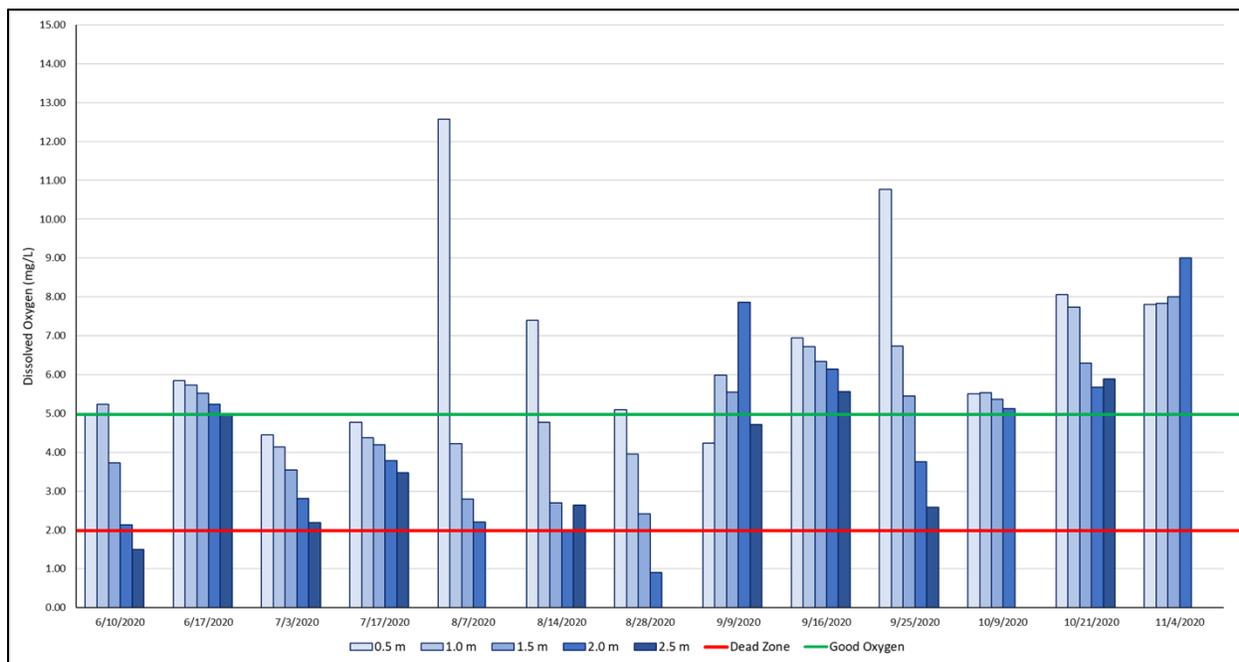
**Figure 2. Dissolved oxygen levels through the water column at Back Creek #1.**
