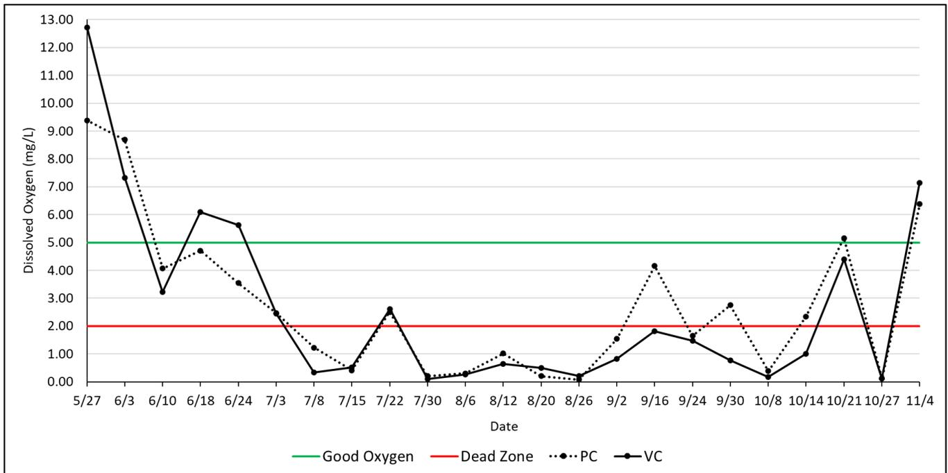
**Figure 4. Bottom dissolved oxygen measured at Plum and Valentine Creek stations in 2020.**
