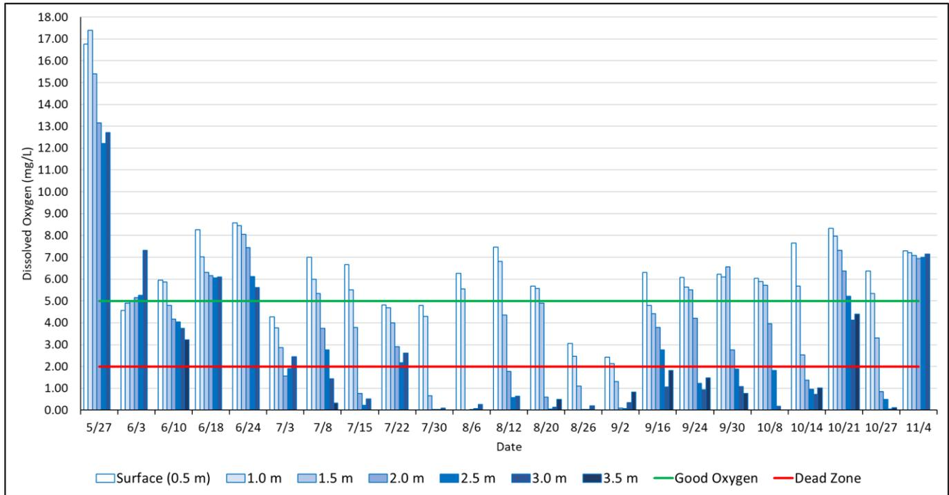
**Figure 3. Dissolved oxygen levels through the water column at Valentine Creek (VC) in 2020.**
